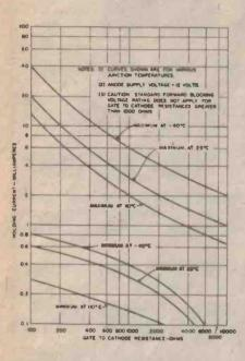
Graph 4. Maximum and Minimum Holding Current Variation with External Gate-to-Cathode Resistance.
