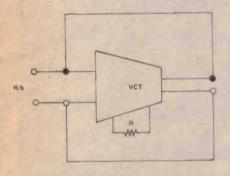
Fig. 4. VCT as a simple resistor.
