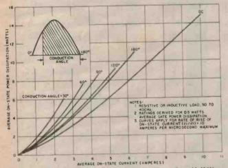
Max. On-State Power Dissipation for Half-Wave Rectified Sine Wave of Current.
