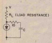
(The 10 ohm resistor limits turn-on current through the SCR to a safe value when the SCR turns on).
