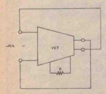
Fig. 5. VCT working as a negative resistance.
