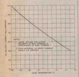
Graph 5. Maximum DC Holding Current vs. Case Temperature.
