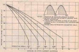
Graph 2. Max. Allowable Case Temperature For Full-Wave Rectified Sine Wave of Current
