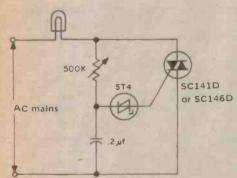
This circuit uses the ST4 IC to trigger the triac (see p105 for data on this device). The ST4 reduces snapon effects that occur in symmetrical trigger circuits and minimizes control circuit hysteresis. This performance is possible with a single RC time constant, whereas a symmetrical circuit of comparable performance would require at lease three additional passive components.
