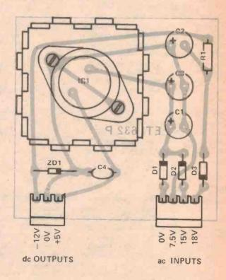
Fig. 6. Component overlay of the power supply board.
