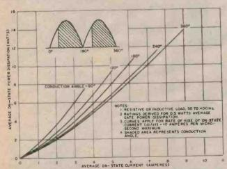
Max. Allowable On-State Power Dissipation for Graph 7. Full-Wave Sine Wave of Current
