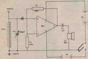
The figure shows how to wire an opamp so that it amplifies the voltage generated across a tuned circuit in order for the circuit to operate as a simple radio receiver. The '741' op-amp is suitable.
