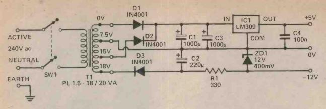
Fig. 3. Circuit diagram of the power supply.
