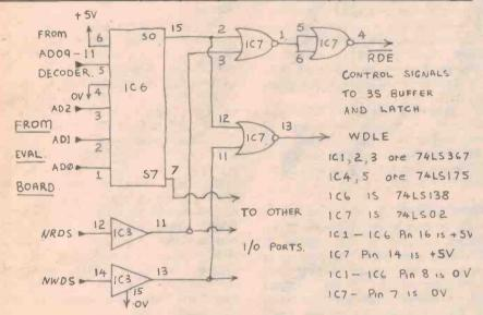
Circuit diagram of 1/0 port, address decoder shown above, data buffers shown below.
