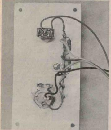
The 'quizmaster's' unit. The three wires connected to the tag-strip go to all the remote 'contestants' units. The other two wires go to the battery.
