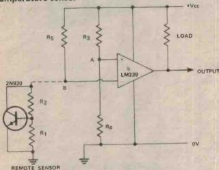
The circuit shows a temperature sensing device which can be used to indicate at a remote point when the temperature passes through a certain value or to give an alarm when this occurs.
